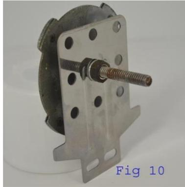
In this case the stud fit through the ¼ inch hole in the adaptor plate. If it hadn't the hole can easily be opened to the appropriate size with a drill. In Figure 10 there is a nut on both sides of the adaptor plate. This allows the badge to be moved in and out to match the depth of the other badges. A lock washer between the nut and adaptor lets you lock it in place.
